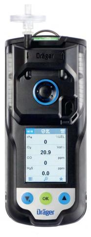
Glowing green D-light indicates that the unit is tested and ready for use
