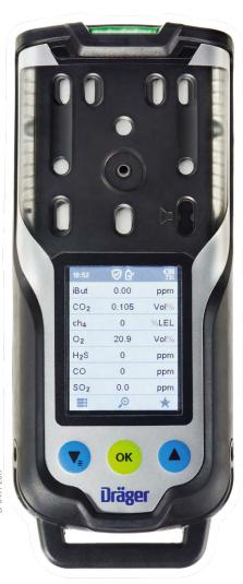
Glowing green D-light indicates that the unit is tested and ready for use
